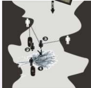
Above: A group pauses during training to grab a bite of lunch. Right: illustration of a typical river rescue exercise covered in the course Manual and practised on the river. This shows several ways of saving someone from a strainer or tree lying in the river.
